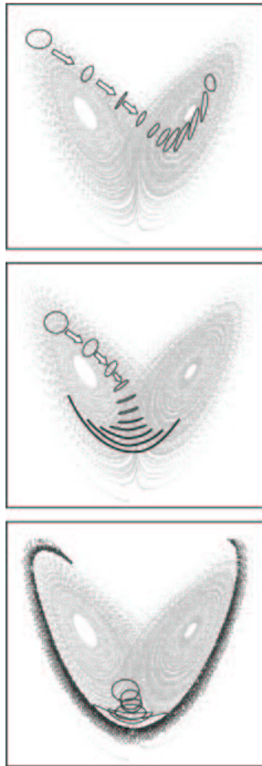
Figure 2: Phase-space evolution of an ensemble of initial points on the Lorenz (1963) attractor, for three different sets of initial conditions. Predictability is a function of initial state.
